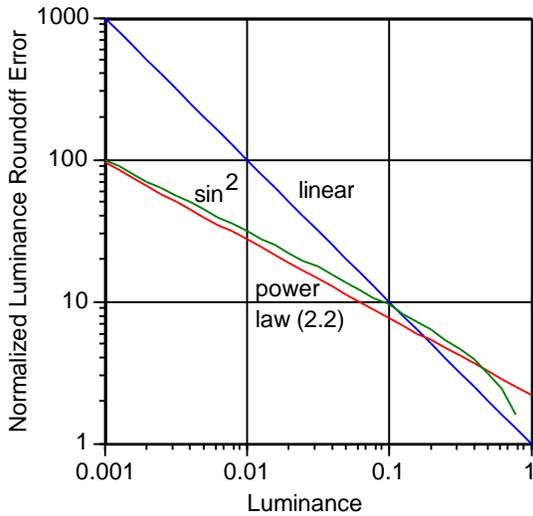
Figure 12: Luminance roundoff error for several device characteristics.
