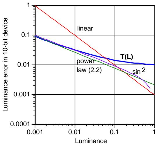
Figure 13: 10-bit device luminance errors compared to the human visual step tolerance,  $T(L)$ .
