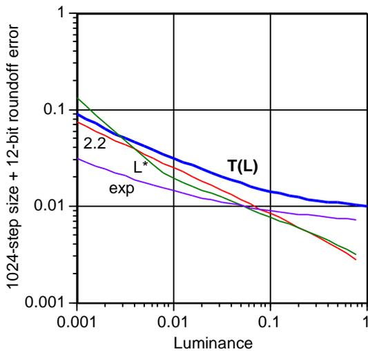
Figure 15: Combined luminance jumps for several 1024-step scales on a 12-bit sin-squared device, compared to visual step tolerance  $T(L)$ .
